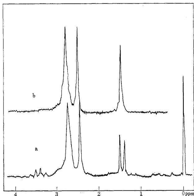
Figure 2.—Pmr spectra for \text{Co}(\text{en})_2(\text{N-Me-L-ala})^{2+} in \text{D}_2\text{O} (a) and for the deuterated complex at the \alpha proton in \text{D}_2\text{O} after treatment with \text{OD}^- (b).
